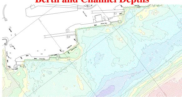
Following a hydrographic survey of the Port and it's approaches on 9<sup>th</sup> August 2023, the below should be regarded as minimum depths by any mariners visiting the port:
